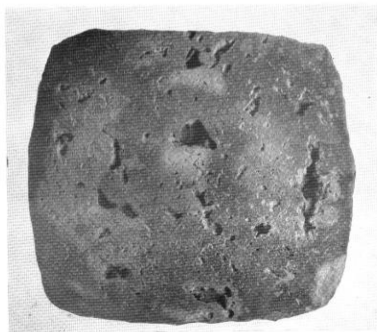
Fig. 6. SECTION AFTER ETCHING, SHOWING POROUS NATURE OF THE IRON. \times \frac{1}{3} approx.
