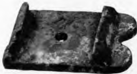
Fig. 2. EARLY PATTERN RAIL with "E.V." Fig. 3. CURVED RAIL, p. 85. Fig. 4. CHAIR WITH HOLE FOR SPIKE, p. 81.
