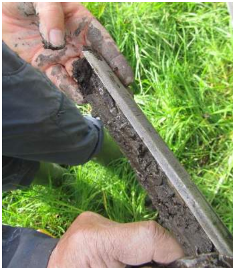
Plate 11.3a. A core containing peat at the base
