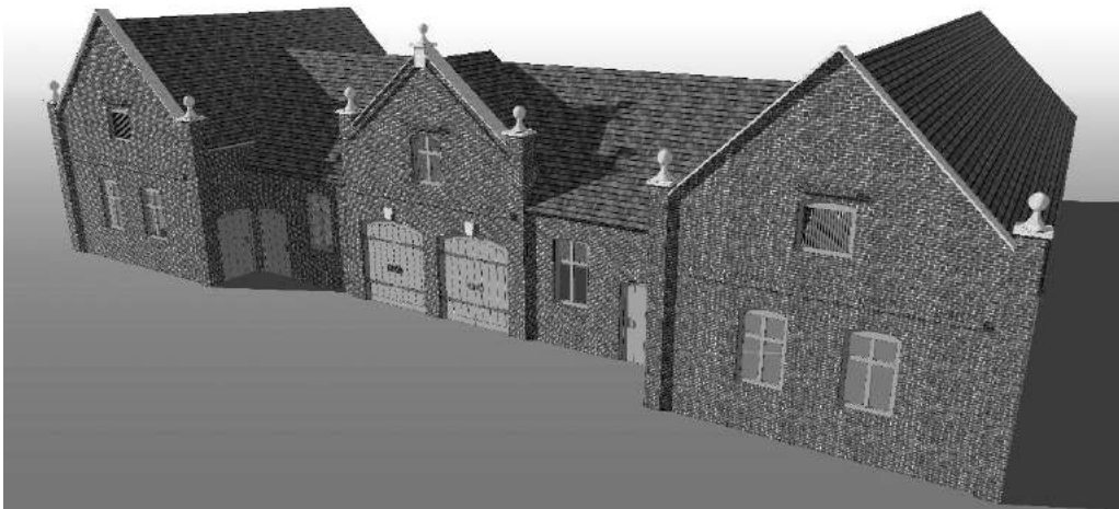
Figure 20. A reconstruction drawing of the building before its conversion to domestic use. Although only one pinnacle with a sphere survives it is likely that the six corner piers were decorated in a similar way
