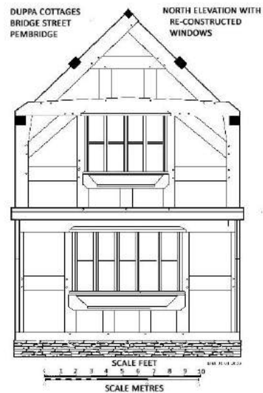
Figure 9. A reconstruction drawing of the jettied north elevation showing the likely form of the two planted-on windows
