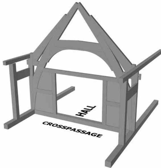
Figure 7. A reconstruction sketch of the spere truss and crosspassage position in Hacton Cruck cottage seen from the south.
