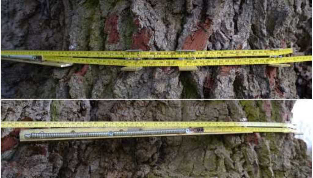
Plate 1.12. The measurement tape in place; note that it sits in a horizontal plane. Readings over two years gave a growth rate of 12.5mm a year
