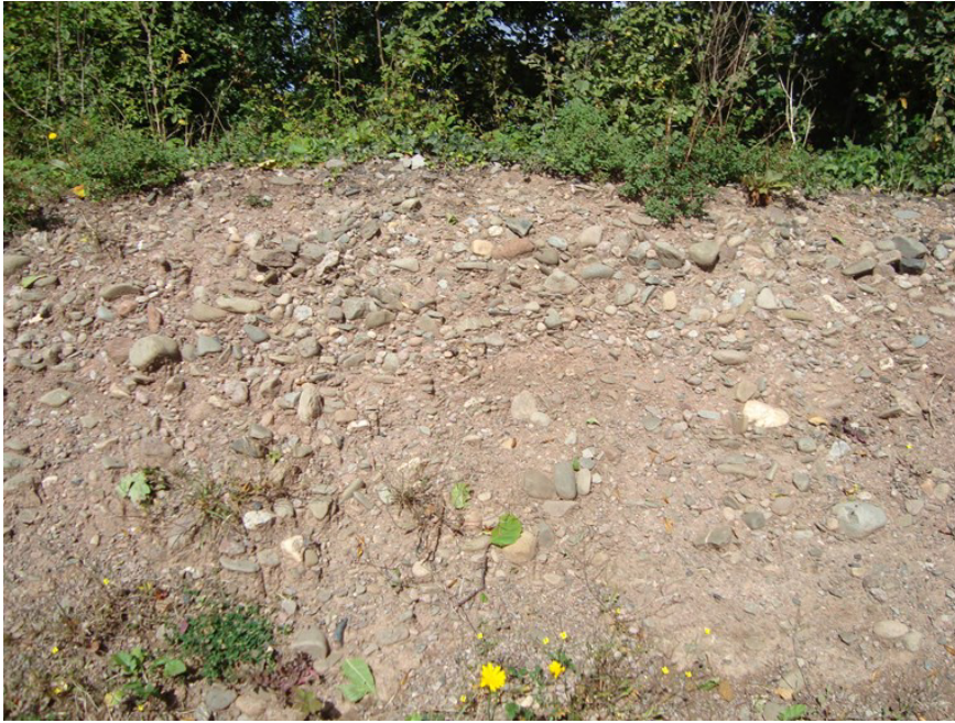
Heterogeneous mix of gravel, sand and clay from the Staunton moraine used as fill for the railway embankment.
