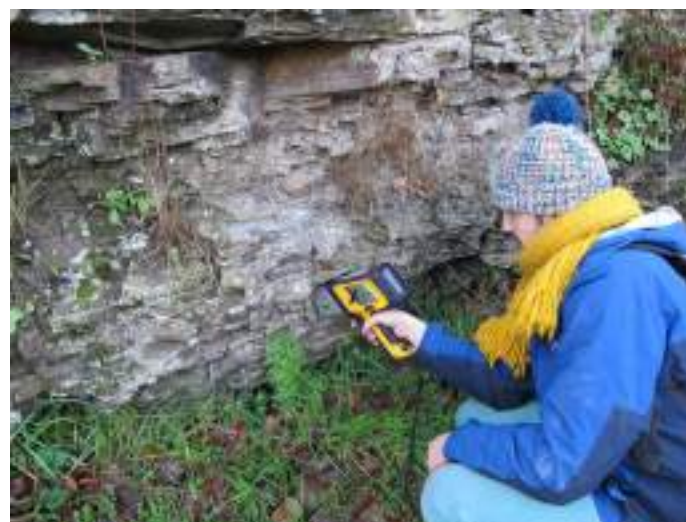
Figure 1 The hand-held X-ray fluoroscope in use
