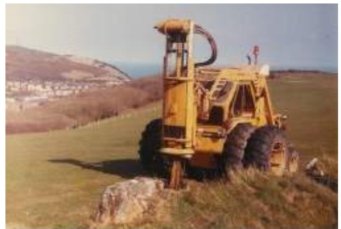
Figure 2 – One method of producing the seismic 'shot'. Here a weight-drop device (Thumper) is employed across a golf course on the Isle of Wight. No 'shots' were acquired from the greens!
