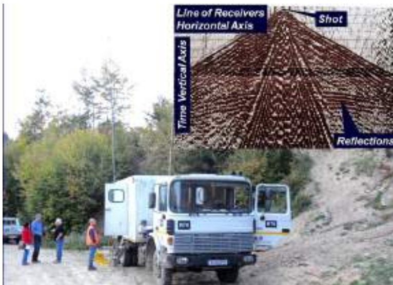
Figure 3 – A recording truck running an onshore survey in Romania. The inset (top right) shows a single shot monitor record.
