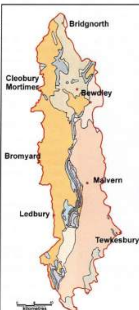
Sketch of the Geopark geological map, showing the complex, North-South Malvern axis with wide areas of uniform Devonian and Triassic rocks to West and East respectively and Carboniferous rocks in the North.
