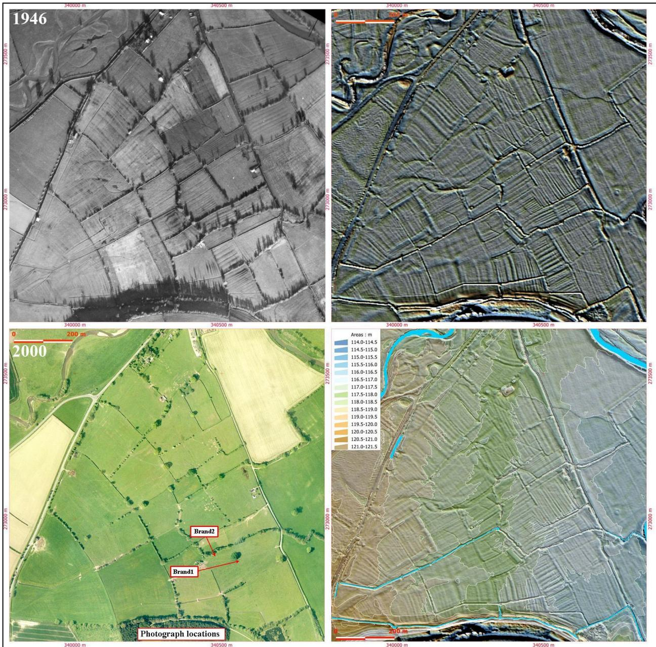
The Brandon to Leintwardine triangle: top left RAF air photo 4th December 1946, top right the differential DTM showing that the meadow earthworks have remained intact since then. Bottom left: air photo 2000 and photo locations (next page), bottom right 50 cm contours derived from the DTM showing the slight slope and drainage to the west.
