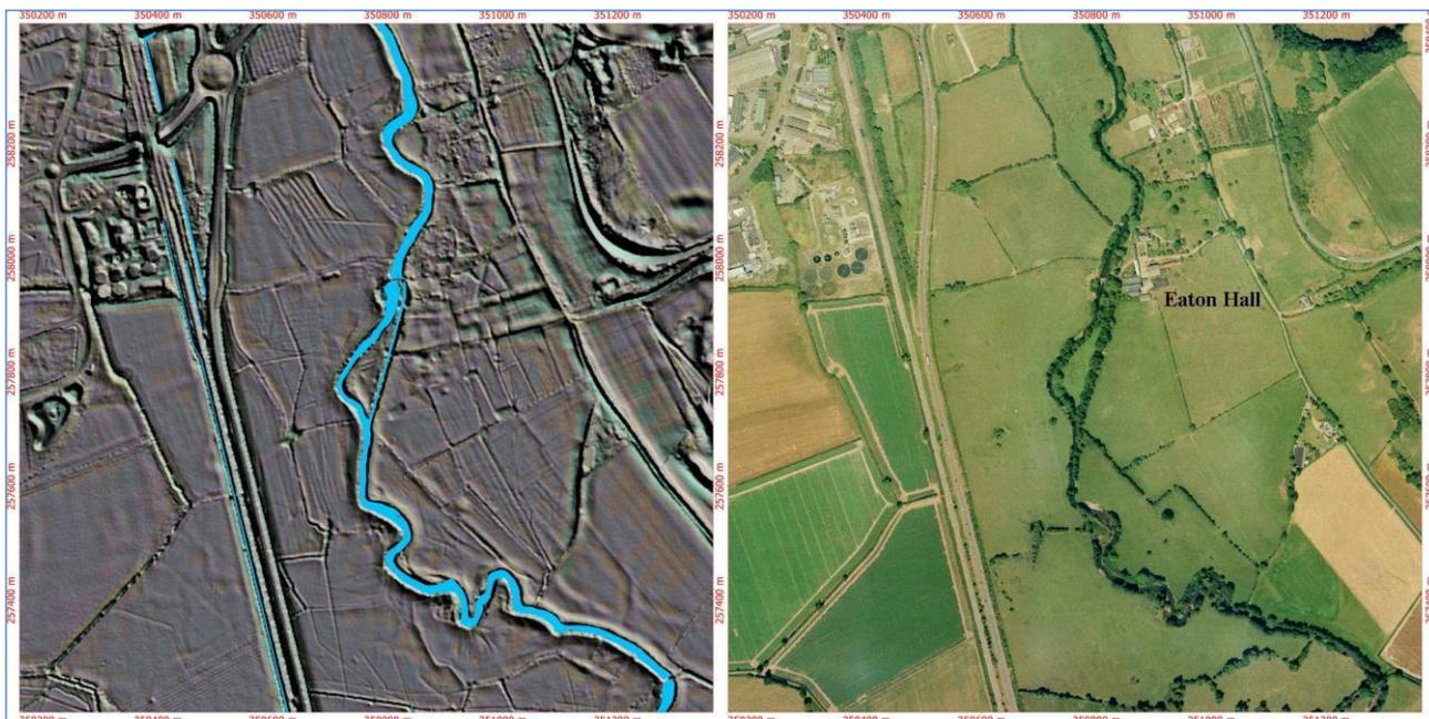
Left: Differential DTM scan showing a complex of channels, meadow irrigation ridges and more modern drainage on either side of the river Lugg but confirming the above field work above referenced. Right: 2000 air photo of same area.
