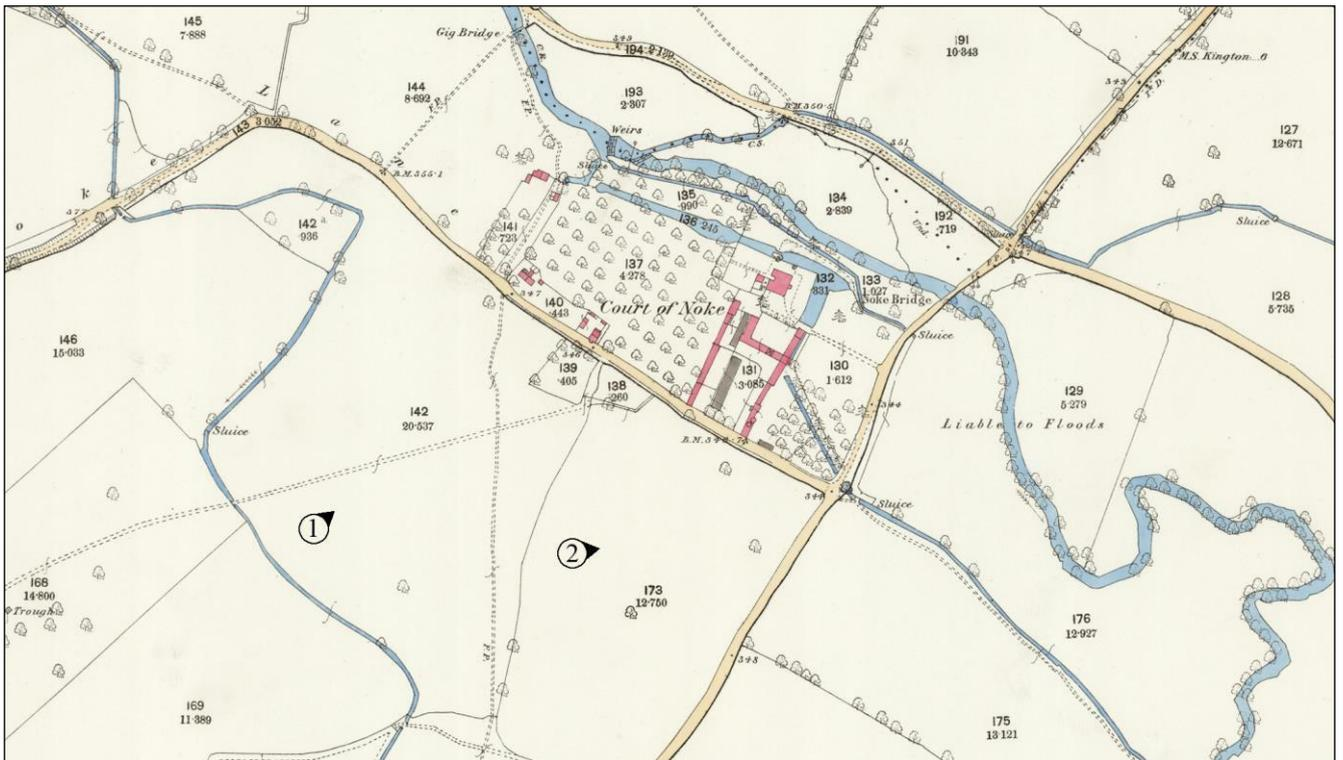
1<sup>st</sup> edition 25' to mile OS map of the Court of Noke showing the two weirs just to the NE, one which controls the water to the channel flowing north east to the land of the Leen and the other through the Court of Noke, augementing the mill tail leat to irrigate the meadows to the east. The two fields opposite and south of the Noke with the photos (above) are irrigated from the main southern channel to the west as it flows along the contours around the hill.
