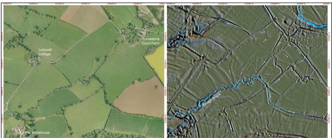
Fields between the Whitehouse and Turnastone Court Farm occupied by Rowland Vaughan from the late 1590s. Air photo from 2000 and DTM render showing a complex of channels and ridges
