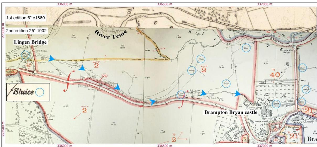
The water carrier channel from Lingen bridge flowing eastwards to Brampton Bryan and the subsidiary channels. Note also the three sluices controlling water to the
