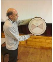
The device may be described as a single function slide rule but (unlike a logarithmic slide rule) the scalar progressions are each linear. So in other words, it is an automated 'subtractor' that reads off instantaneous heights above sea level - when set up and given the appropriate data.
