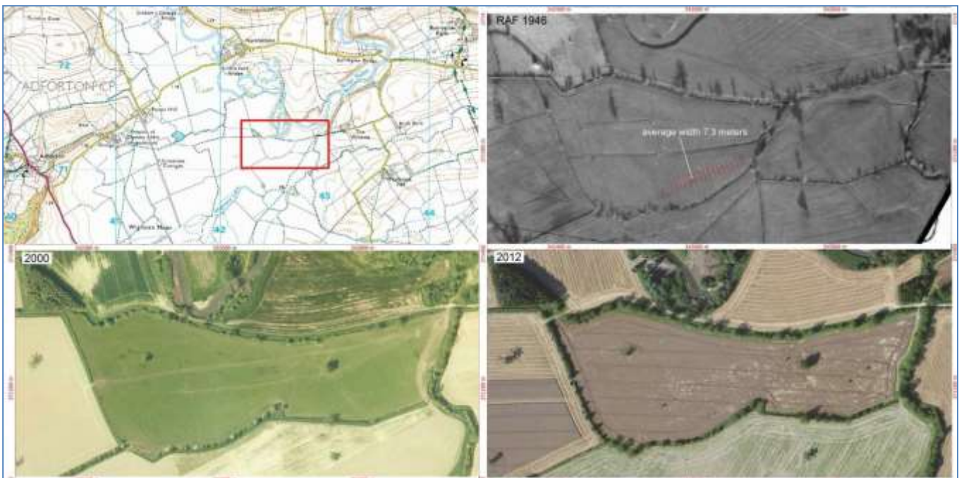
Water meadow site HER 41910 (Water meadow, Willows Farm). Top right: on the December 1946 RAF air photo the bedworks are fairly evident with a mean width of 7.3m the 2000 aerial photograph also shows up the ridges/panes even though the photo is taken in summer and field appears as permanent pasture probably not ploughed since the earthworks are prominent enough to be recorded as HER site. However by 2012 the whole field is in arable cultivation.
